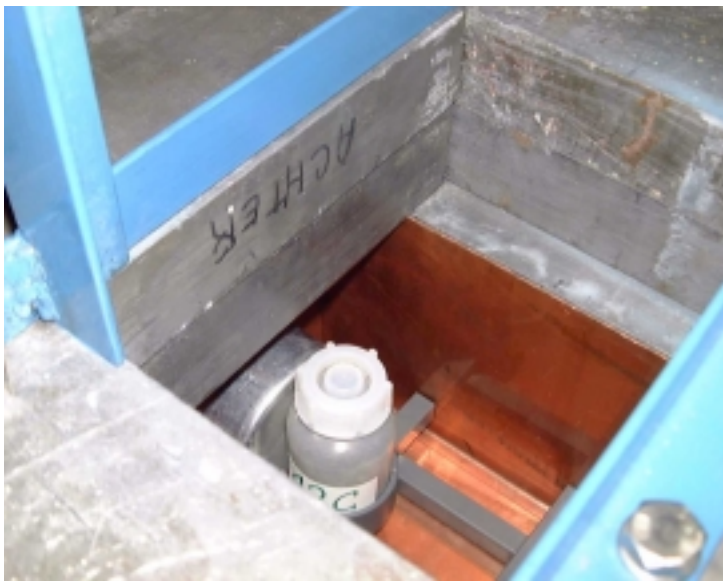
Fig. 4: a sample in front of the detector inside the shielding
